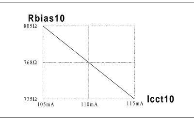
Figure 11. RBIAS10 Resistance versus I<sub>CCT10</sub>
